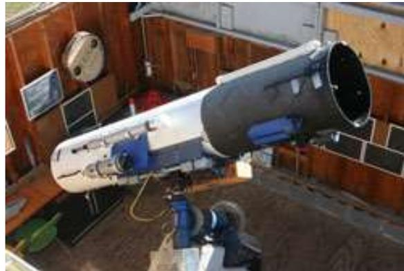
The first telescope installed at Indian Hill. A 16 inch F7 classical Newtonian Reflector on a German Equatorial Mount. Computer controlled, electric focuser, and autoguider capabilities.
