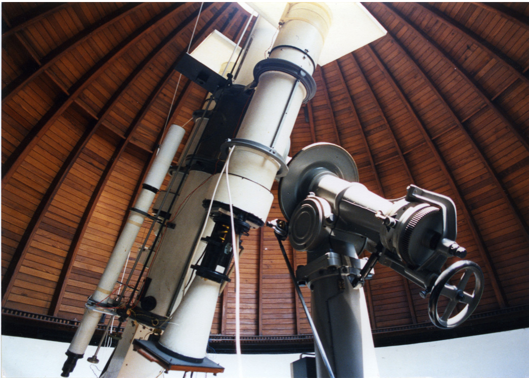
Photo-visual Zeiss refractor used in the discovery of 1700 Zvezdara. The photograph shows the telescope after it had been set up for use with a spectrophotometer in the early 1970s.
